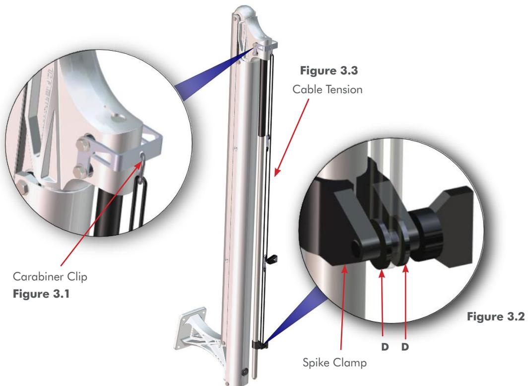
**NOTE:** Before tightening wing screw, make sure to keep Downrigger cables tight as shown in FIG. 3.3
