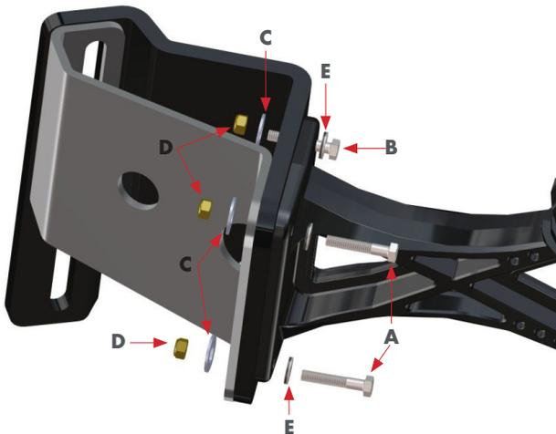
**NOTICE:** Ensure Neo-Bond side of washer is facing the Stern Bracket.
